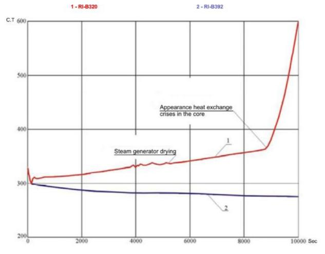
Figure 29 – Maximum temperature of fuel element cover at full loss of alternative current sources
