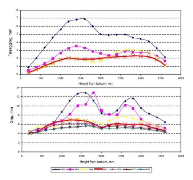
Figure 15 – Changing of bends and inter cassettes clearances in plant 1 at increasing FA-2 in the area
