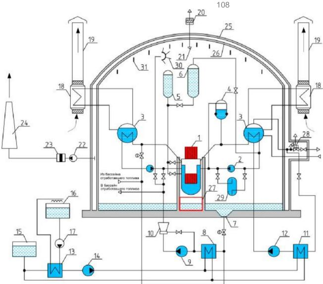
Figure 26 – Energy unit safety system diagram
