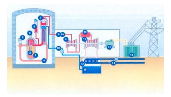
(1) reactor, (2) core, (3) absorbing rod, (4) primary cooling circuit, (5) main circulating pump, (6) pressure compensator, (7) steam generator, (8) secondary cooling circuit, (8a) steam for turbine, (8b) water for steam generators, (9) high-pressure cylinder, (10) steam superheater, (11) low-pressure cylinder, (12) generator, (13) condenser, (14) condenser cooling water circuit, (15) condensate, (16) transformer.
