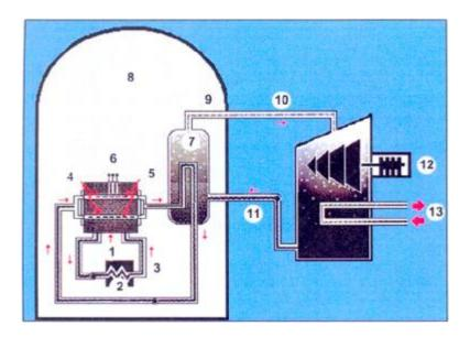
(1) reactor, (2) heat exchanger, (3) moderator, (4) fuel channels, (5) fuel, (6) control rod, (7) steam generator, (8) protective containment, (9) steam, (10) steam line, (11) pump, (12) turbine generator, (13) water for a condenser cooling.
