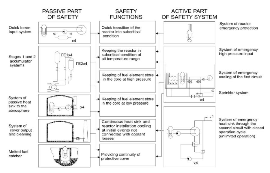
Figure 27 – Basic solutions on providing safety functions in project NPP-92
