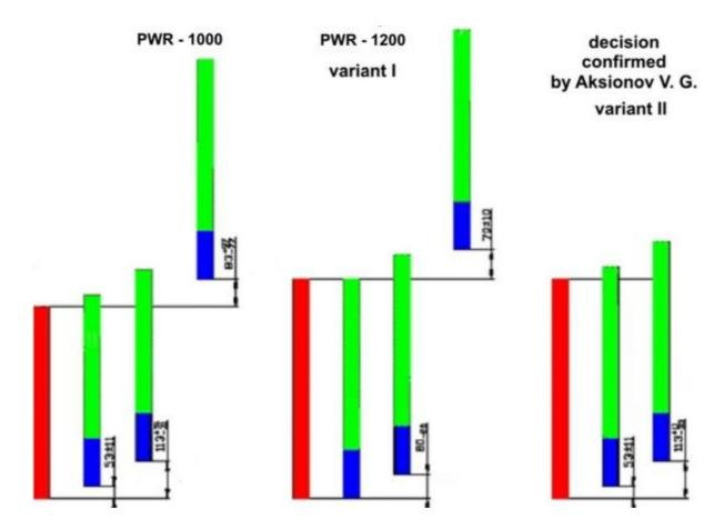
Figure 18 – Relative positions of fuel and absorber
