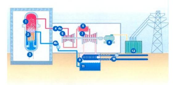
(1) reactor, (2) core, (3) absorbing rods, (4) primary cooling circuit, (4a) steam for turbine, (4b) water for reactor, (5) high-pressure cylinder, (6) steam superheater, (7) low-pressure cylinder, (8) generator, (9) condenser, (10) cooling water circuit, (11) condensate, (12) transformer.
