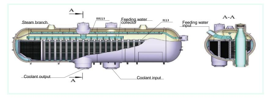
Figure 23 – Longitudinal section of a steam generator
