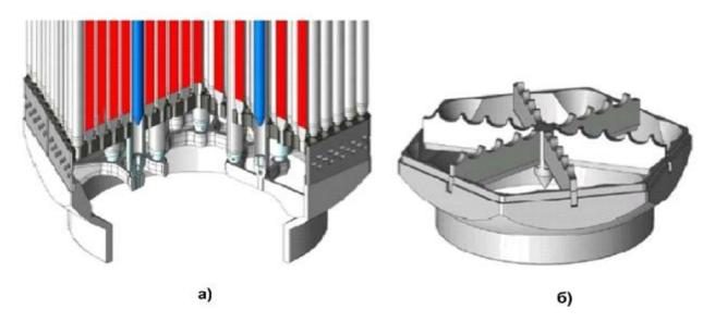
Figure 17 – Shank end with long NK a) and standard FA-2M shaft end δ)
