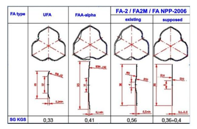
Figure 12 – SH cells of different FA types
