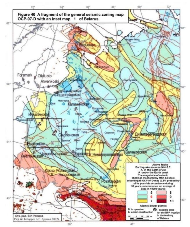
Figure 40 – Map fragment of the seismic risk zoning OSR-97-D with insert (1) of the map of Belarus.
